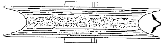
PULLEY NOT ALIGNED CORRECTLY
