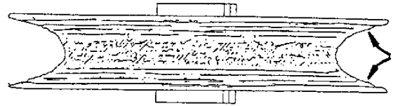
PULLEY NOT ALIGNED CORRECTLY
