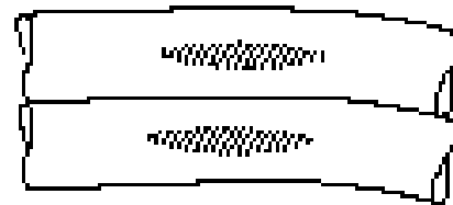
EACH OUTER WIRE WORN LESS THAN 40% (WORN AREAS NOT BLENDED)
